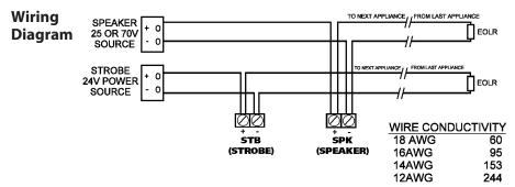
\* MAX. WIRE DISTANCE (IN FEET) = PANEL VOLTAGE - DEVICE MINIMUM VOLTAGE X WIRE CONDUCTIVITY (STROBE ONLY)
