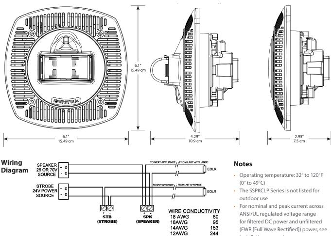
\* MAX. WIRE DISTANCE (IN FEET) = <u>PANEL VOLTAGE - DEVICE MINIMUM VOLTAGE</u> x WIRE CONDUCTIVITY (STROBE ONLY) TOTAL CURRENT DRAW
