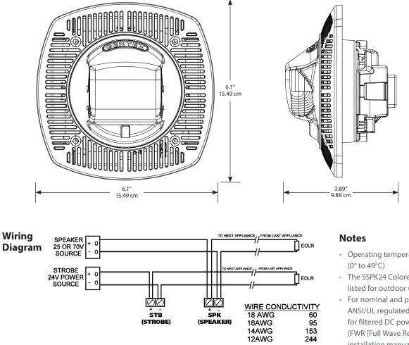
\* MAX. WIRE DISTANCE (IN FEET) = <u>PANEL VOLTAGE - DEVICE MINIMUM VOLTAGE</u> x WIRE CONDUCTIVITY (STROBE ONLY) TOTAL CURRENT DRAW
