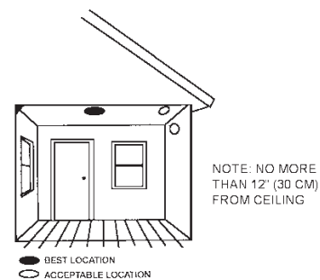
FIGURE 5: RECOMMENDED SMOKE ALARM MOUNTING LOCATIONS.
