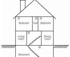
FIGURE 5: A SMOKE ALARM MUST BE LOCATED ON EACH LEVEL IN ADDITION TO EACH BEDROOM.
