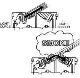
Under normal conditions, the light generated by the pulsing infrared LED is not seen by the light sensor, as it is positioned out of the direct path of the light beam. When smoke enters the sensing chamber, light from the pulsing LED light source is reflected by the smoke particles onto the photodiode light sensor. At the first sighting of smoke, the device is put into a pre-alarm mode. This is indicated by a rapidly flashing red LED on the face of the smoke/CO alarm.
