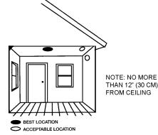
FIGURE 6: RECOMMENDED SMOKE/CO ALARM MOUNTING LOCATIONS
