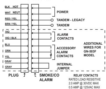
**CAUTION:** RED/YELLOW and BROWN/YELLOW wire to be capped when not in use. This wire is for tandem connection only. DO NOT connect to any other circuit.
