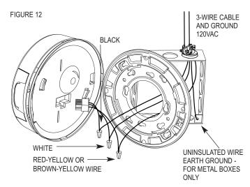
NOTICE: RED-YELLOW WIRE AND BROWN-YELLOW WIRE: THE RED-YELLOW WIRE AND BROWN-YELLOW WIRE FROM THE SMOKE/CO ALARM IS FOR TANDEM CONNECTION ONLY. DO NOT USE, AND DO NOT REMOVE INSULATION CAP UNLESS CONNECTING ANOTHER CO ALARM, SMOKE/CO ALARM OR SMOKE ALARM.
